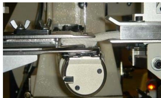
6. Lower plate moves backwards for second fold.
