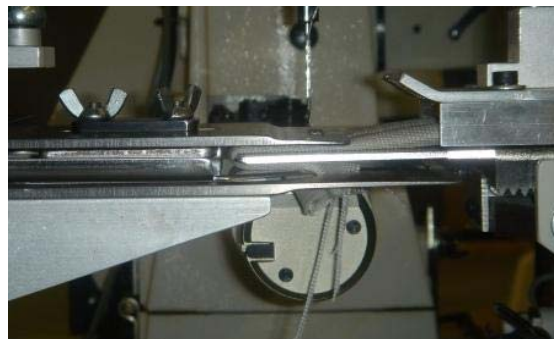
5. Inside plate moves forward for first fold.
